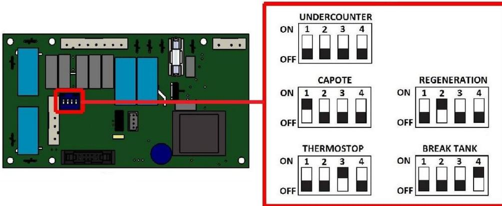
**CAUTION:** DISCONNECT THE MACHINE ELECTRICALLY FROM THE MAIN BREAKER BEFORE ACTIVATING ANY SWITCH.
